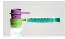
If you add a syringe to the Connector Ring, it is possible to force low pressure to support the straining of rough sample material while pulling the piston.
